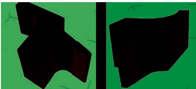
Figure 9(a). X-ray image of seal fin showing coating is uncracked
