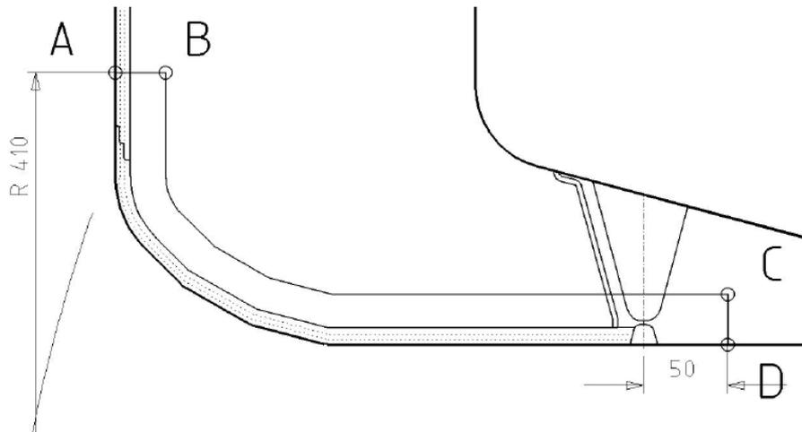
Figure 3. Inspection volume of RPV nozzle inner corner area. Inspection volume marked with A-B-C-D.
