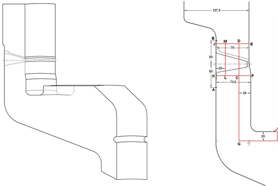
Figure 2. Steam generator collector dissimilar metal weld geometry and inspection target.
