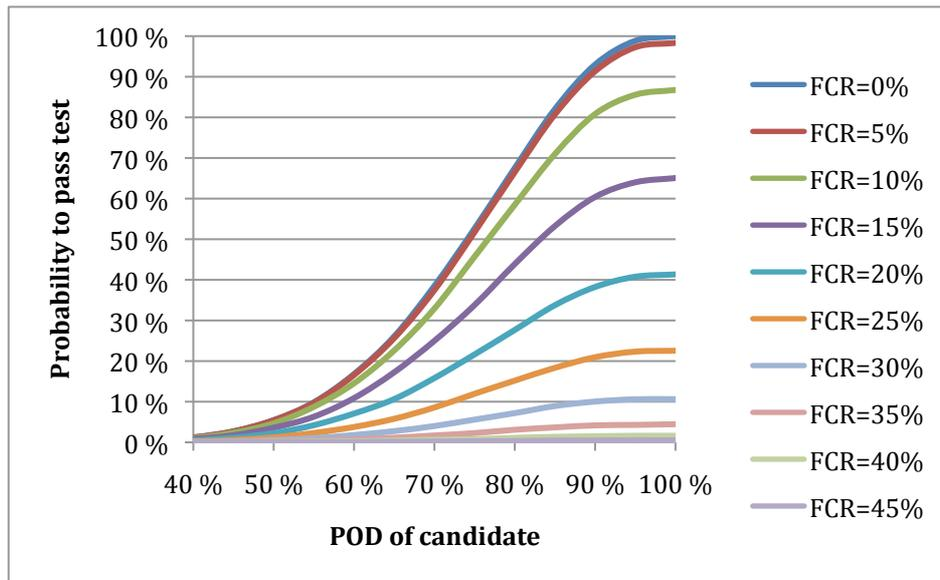
Figure 1. Monte-Carlo simulation for ASME Section XI, Appendix VIII, Supplement 2 detection acceptance criteria (Table VIII-S2-1) with 10 flawed grading units (minimum required). Curves show different false call rates (FCR). Monte-Carlo simulation used 100000 random samples per point (21 million random samples in total).
