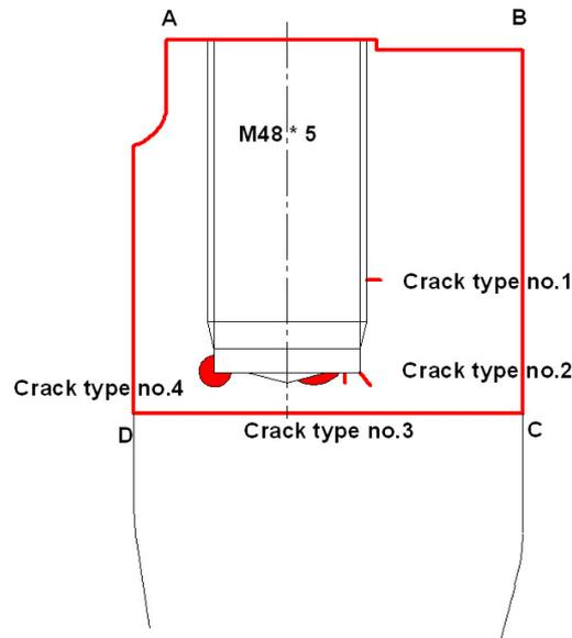
Figure 4. Inspection volume of threaded holes of steam collector flange area (marked A-B-C-D)
