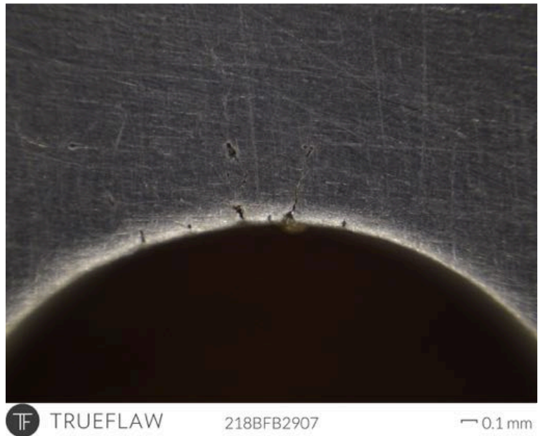
Figure 3. Microscopic image of typical crack in aluminum.
