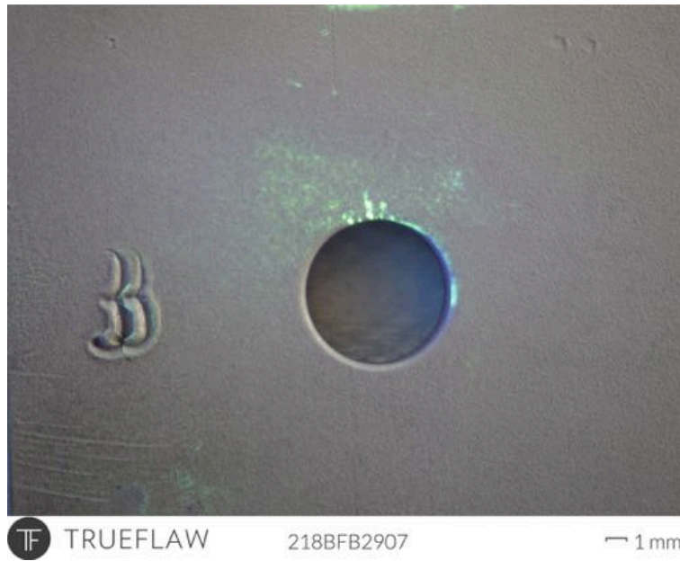
Figure 5. FPI image of typical crack in aluminum. The crack is the same as that depicted in Figure 3 (Trueflaw crack number 218BFB2907).
