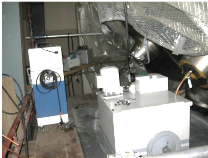
Figure 9. General view from the assembly of the manufacturing system outside of the reactor pressure vessel. In the front right is fluid collector and on the left side behind is the air filter of the local ventilation
