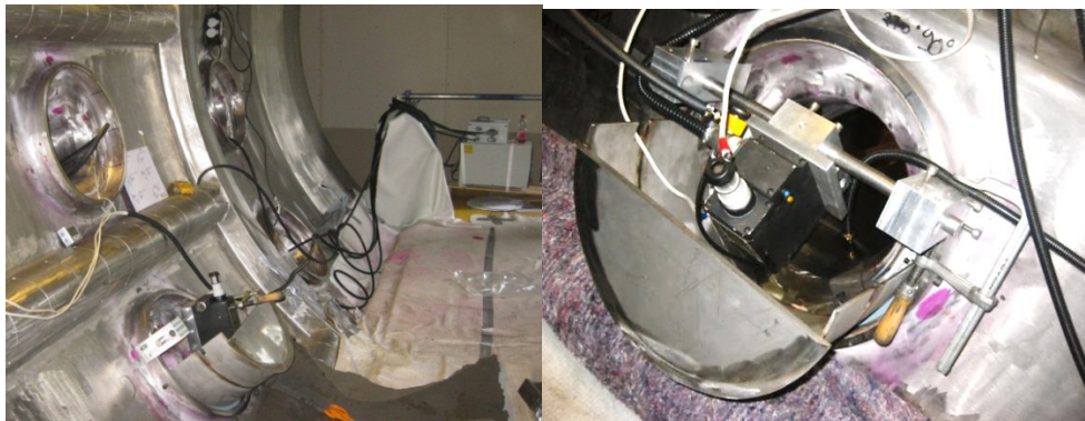
Figure 8. General view from the assembly of the manufacturing system on left and assembly of the EDM machining head on the right
