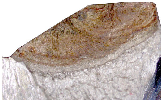
Figure 6. Fracture surface from a destructively examined validation crack corresponding to crack type 3 in Figure 3.
