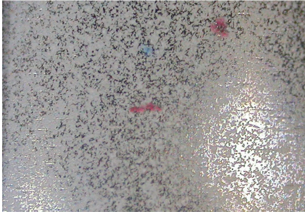
Figure 2 Small crack initiation in Alloy 690 steam generator tube; a dye penetrant indication.
