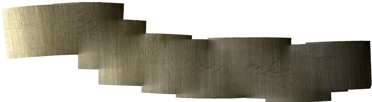
Figure 3 Circumferential cracking in steam generator tube samples.
