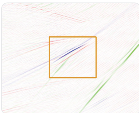
Crack detection from PWI/TFM data
